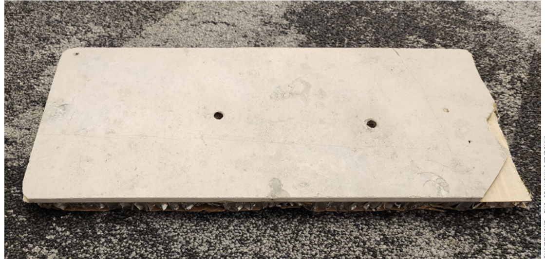
Failed thin stone panel with honeycomb backing.
